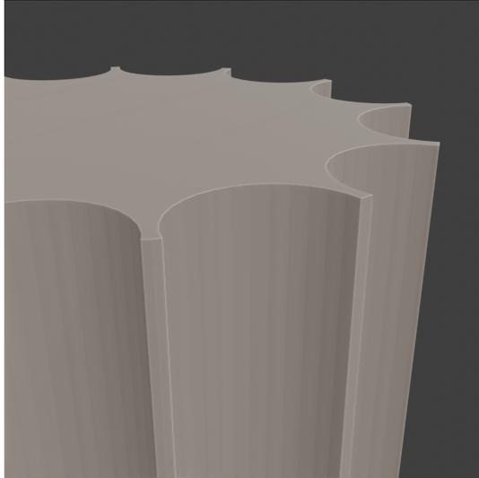
Figure 5: Column generated from  $r = 4, n = 12, v = -0.08, h = 20$ . This figure highlights the blunted edges that occur for negative values of  $v$ , as described in section 2.4
