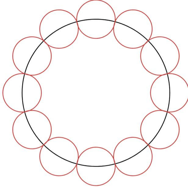
Figure 2: Original cylinder (in black), and the circular pattern of cylinders (in red) that will be cut from it.
