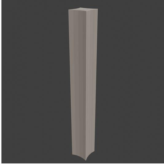
Figure 7: Column generated from  $r = 4, n = 4, v = 0.01, h = 20$ . Large parts of the base cylinder are cut when small  $n$  are used.
